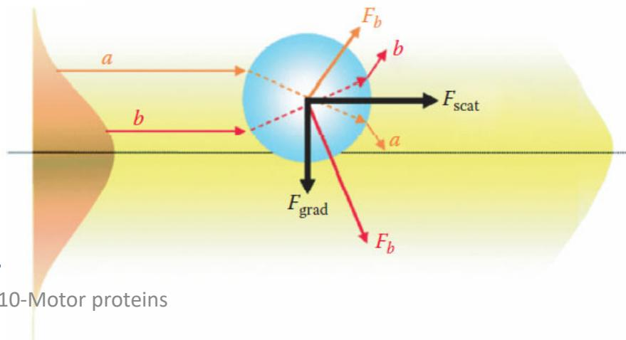
Particle with diameter  $d$  in laser beam with gaussian profile
